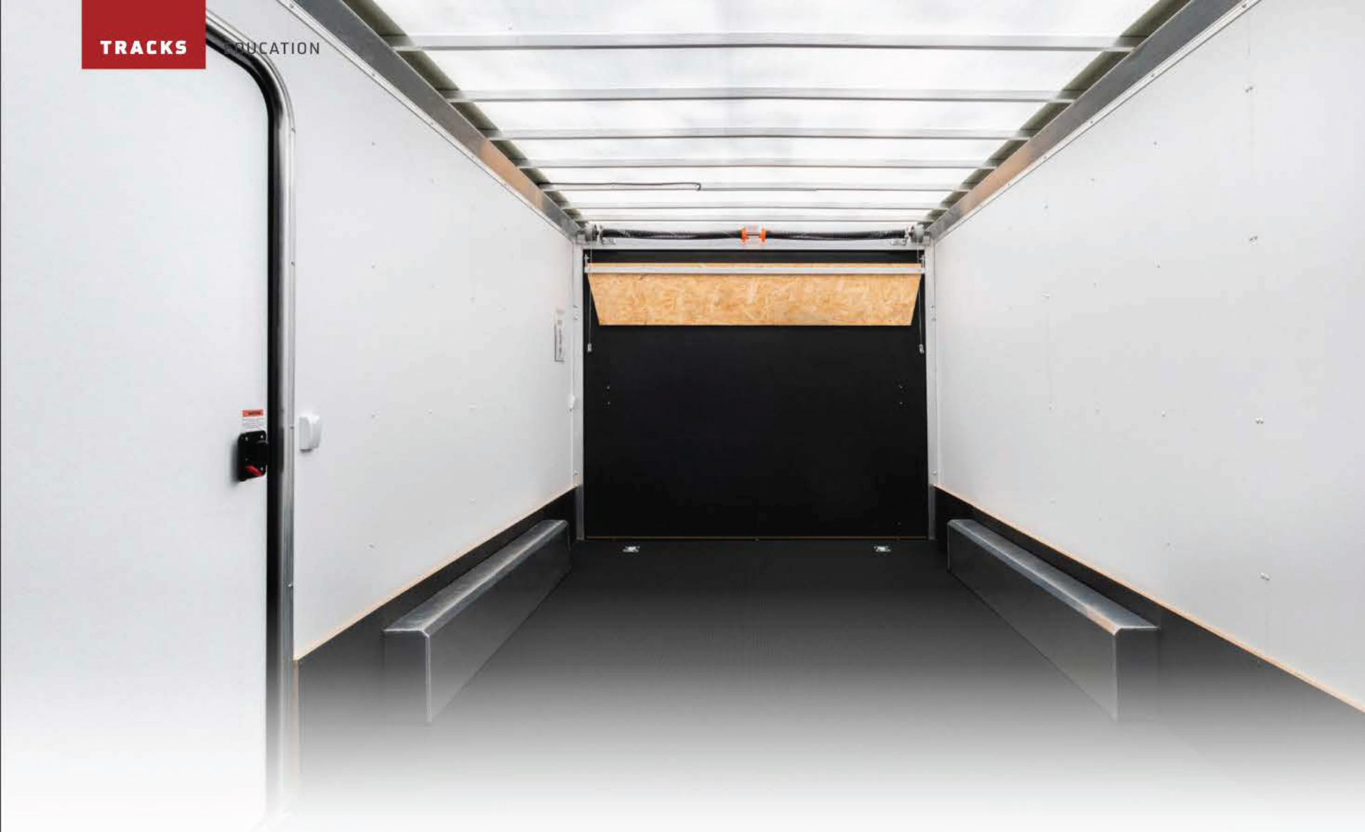
The LIGHTLID Roof enables natural light inside the trailer for better visibility while retaining durability and weather resistance. Photo provided by UFP Factory Built Cargo.
